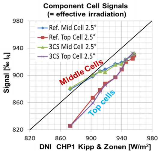
**FIGURE 4.** Component cell signals from two different sensors compared to the DNI measured by a CHP1 Kipp & Zonen pyrheliometer. All sensors have a  $2.5^\circ$  field of view half angle.
