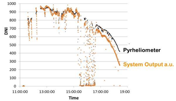
**FIGURE 5.** CPV system output compared to DNI.
