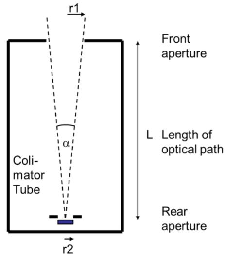
FIGURE 1. Basic design of a direct light sensor
