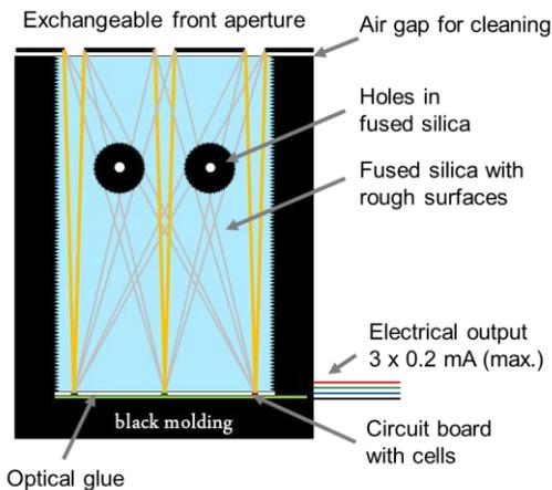
**FIGURE 2.** The 3CS direct irradiation sensor
