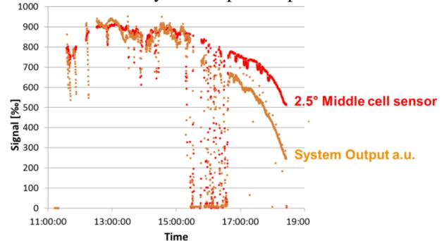
**FIGURE 6.** CPV system output compared to 3CS middle cell sensor with  $2.5^\circ$  opening half angle.
