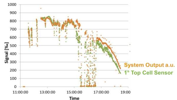
**FIGURE 8.** CPV system output compared to 3CS top cell sensor with  $1^\circ$  opening half angle
