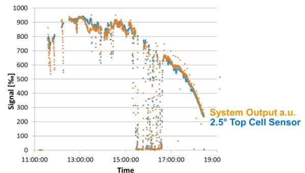
**FIGURE 7.** CPV system output compared to 3CS top cell sensor with  $2.5^\circ$  opening half angle
