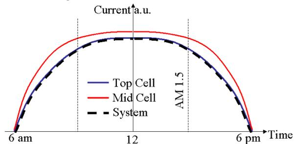
**FIGURE 10.** A CPV system with too little blue response is always top cell limited.
