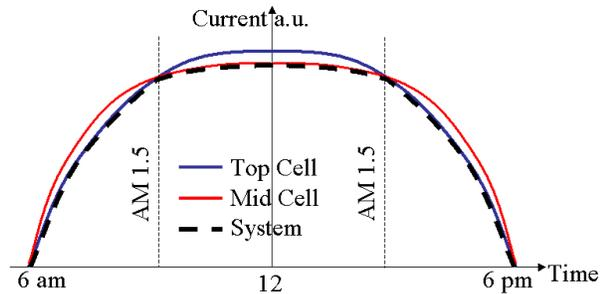
**FIGURE 9.** A balanced CPV system is top cell limited in the morning and evening and middle cell limited at noon.
