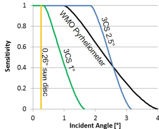
**FIGURE 3.** Angular sensitivity of the 3CS with different apertures in comparison to a WMO standard pyrheliometer
